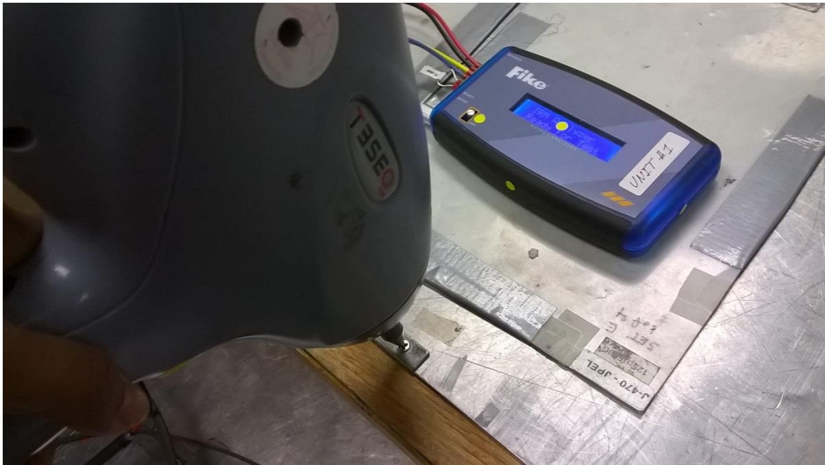
Figure 9 - ESD, Horizontal Coupling plane
