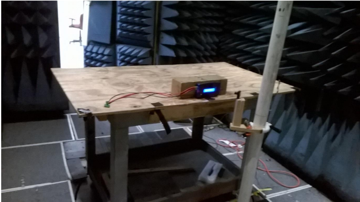
Figure 11 - Radiated Immunity Test Setup, Side A All six sides have been tested in similar fashion
