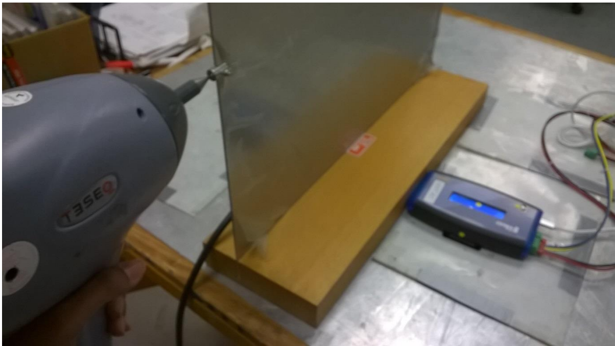
Figure 10 - ESD, Vertical Coupling plane
