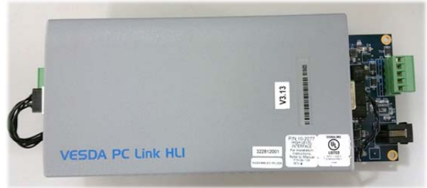
Figure 1 – Fike PC Link HLI Assembly
