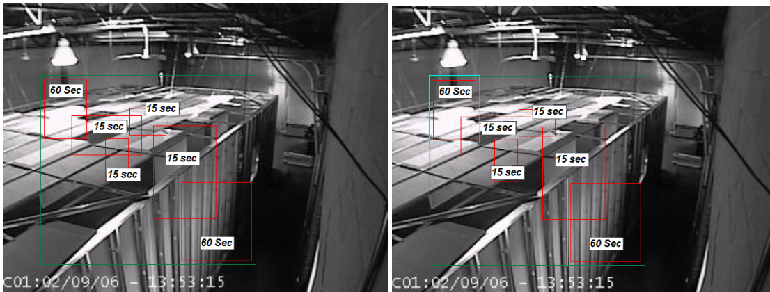
Fig 20 – Two 60 second events connected by a string of four 15 second events. Branch 1 results in a single zone (Green) encompassing all events with no delay. Branch 2 results in two smaller zones (light blue) encompassing the 60 events with the string of 15 seconds events eliminated due to a 15 second delay. The zone area of Branch 2 is smaller so that is the chosen solution.
