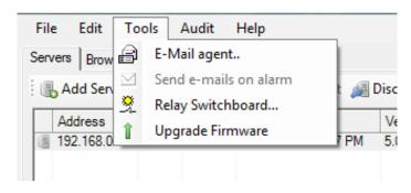
Within the Relay Switchboard window (see below) you will find two tabs. The features within each tab will allow you to generate new rules, arrange the order of the rules, edit rules, delete rules, and test relay functionality. Initially the rules list will be empty. In order to populate the list, right-click within the list box and select *New rule* or click the *New Rule* button. In response the Video Analytics software will open the *Relay Rule Wizard*.
