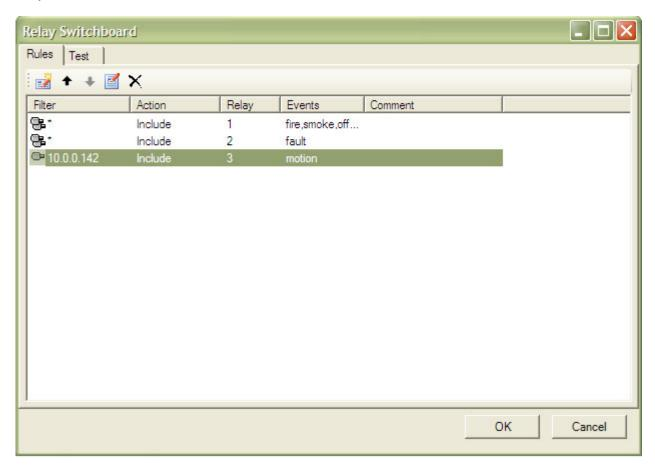
You may test the relay engagement by using the *Test* tab where each relay can be engaged/disengaged manually using the proper checkbox.
