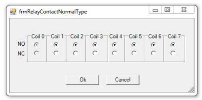
NOTE: Should power to the Wise relay module be lost, all relay contacts will default to the normally open state.
