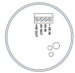
The Loop +ve (positive) IN and the Loop +ve (positive) OUT connections are split within the module, for cable continuity readings at the commissioning stage they must be temporarily removed and connected through. Please remember that all high voltage testing must be carried out before the installation of the electronics, otherwise the electronics will be damaged. Please also remember to use a suitable connection (not supplied) to maintain the screen integrity of the loop.
