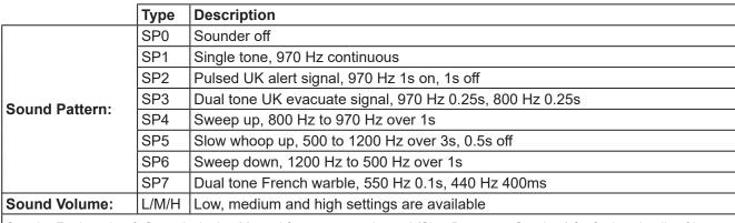
See the Engineering & Commissioning Manual for your control panel (Sita, Duonet or Quadnet) for further details of how to program the above.
