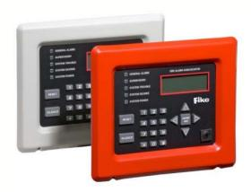
The FIK-RA1000R can be surface or flush-mounted. Use the optional trim ring for surface mounting. When flush mounting an electrical box is optional. If using an electrical box, use a 4-square, single-gang, or double-gang box.
