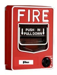
The mechanical operation is simple and easy to use in an emergency with a PUSH IN/PULL DOWN handle that latches in the down position to clearly indicate the station has been operated. Simultaneously, the word "ACTIVATED" appears on top of the handle in bright yellow, further indicating the station's operation.
