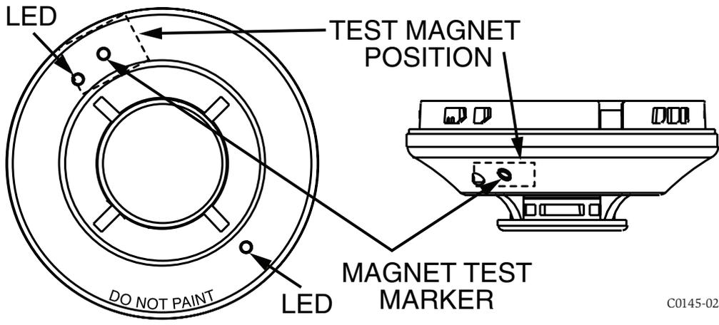
**FIGURE 5. DETECTOR COMPONENTS**
