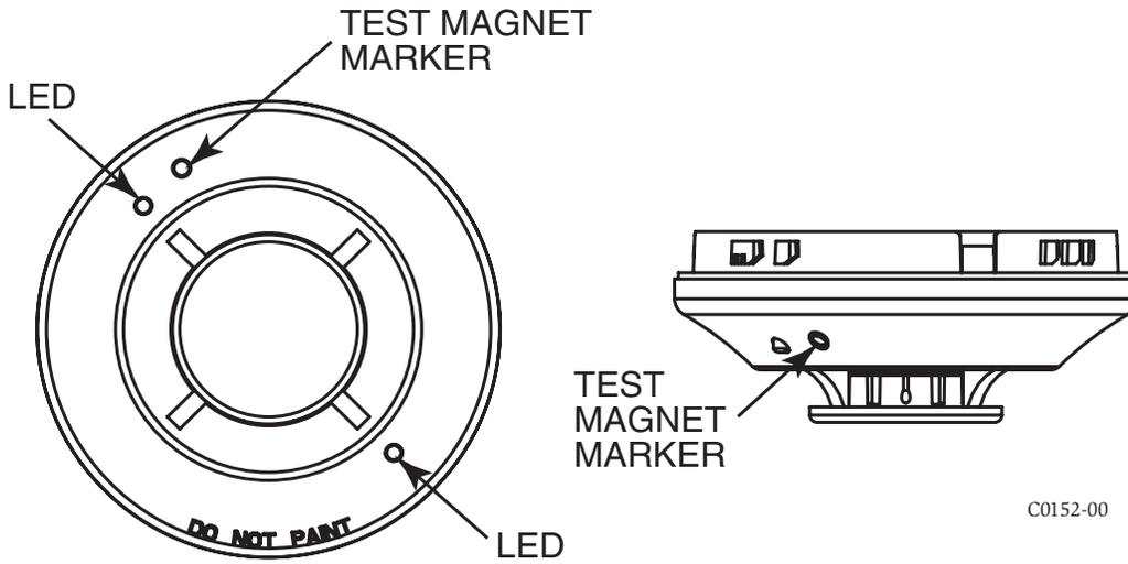
**FIGURE 5. DETECTOR COMPONENTS**
