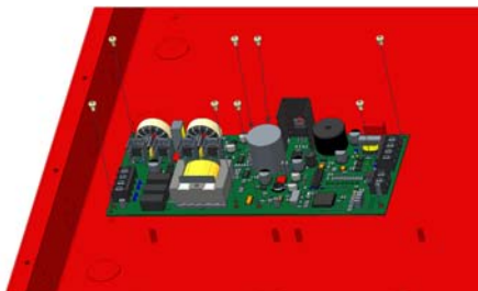
Figure 2 FIK-INT50W in the FACP Cabinet Under The Main Control Board
