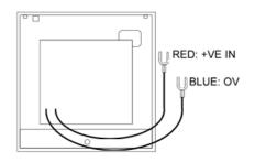
Twinflex Soundpoints can be mixed on the same zone as other types of Twinflex device (eg. Twinflex Multipoint Detectors). The above diagram shows how to make the zone positive, zone negative and screen connections between the control panel and Twinflex Soundpoints. Refer to the instructions of other Twinflex devices for their equivalent wiring/terminal labelling details.
