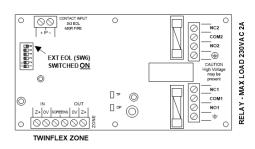
For use as a simple 'change-over' relay output, connect to relay contacts as above, **remembering** to set the External EOL switch to ON.
