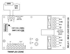
For use as an unmonitored input, connect to input as shown above, remembering to set the External EOL switch to ON.
