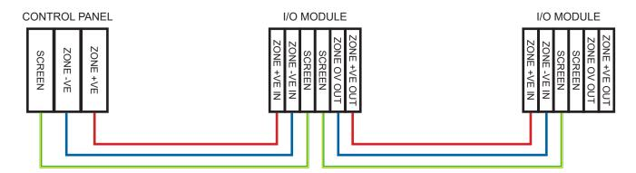
The Twinflex I/O Module can be mixed on the same zone as other types of Twinflex device (eg. Twinflex Multipoint Detectors). The above diagram shows how to make the zone positive, zone negative and screen connections between the control panel and Twinflex I/O Modules. Refer to the instructions of other Twinflex devices for their equivalent wiring/terminal labelling details.
