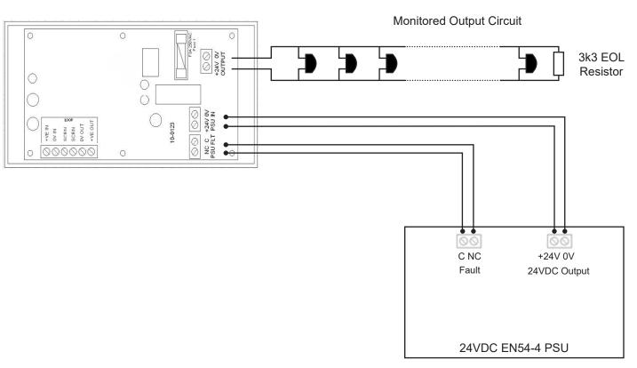
Notes: This module monitors the output circuit only in the quiescent state using a reverse voltage. Any devices connected to the monitored output circuit MUST be polarised and protected from operation if voltage is applied in the reverse polarity. This can normally be achieved by the addition of blocking diodes.
