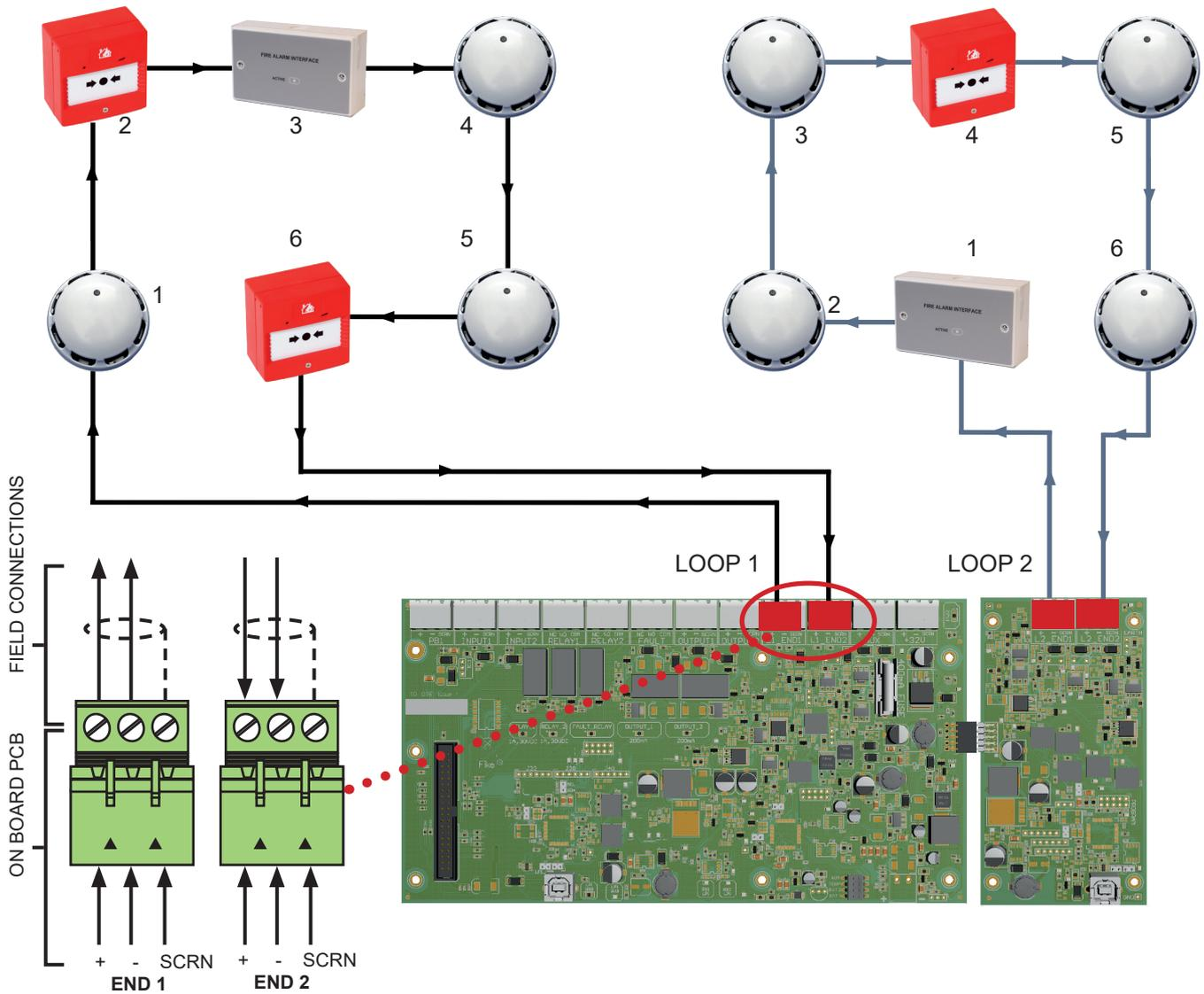
Communications run from Loop End 1 but in the event of a continuity fault (O/C or S/C), communications will be sent from both ends of the loop. So for a single loop fault, no devices will be lost.
