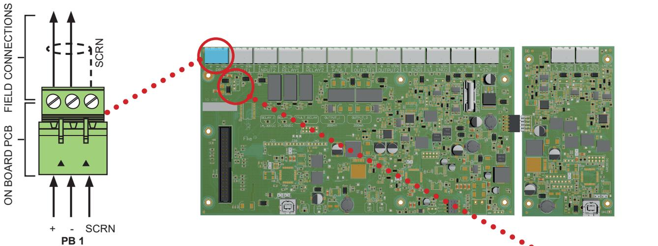
The jumpers are fitted to impedance match the cable with the driver ICs & prevent signal reflections down the cable. The jumpers must be changed on the CIE and last RDU.
