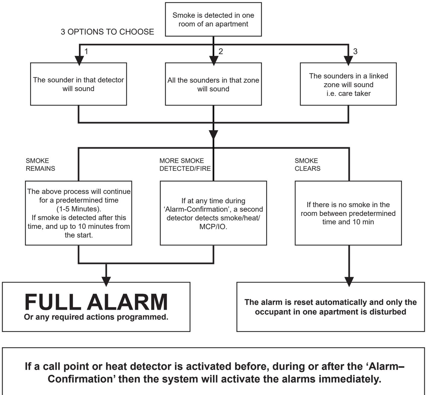
This function affects the smoke detector only, and operates before the control panel enters the fire state. Thus, the system 'Cause & Effect' does not need to be adjusted as **Alarm Confirmation takes place before the programmed Cause & Effect sequence is reached.**
