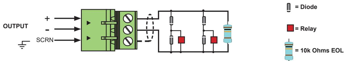
The default setting for Output 1 is a Sounder Output and the default setting for Output 2 is a Common Fire Output.
