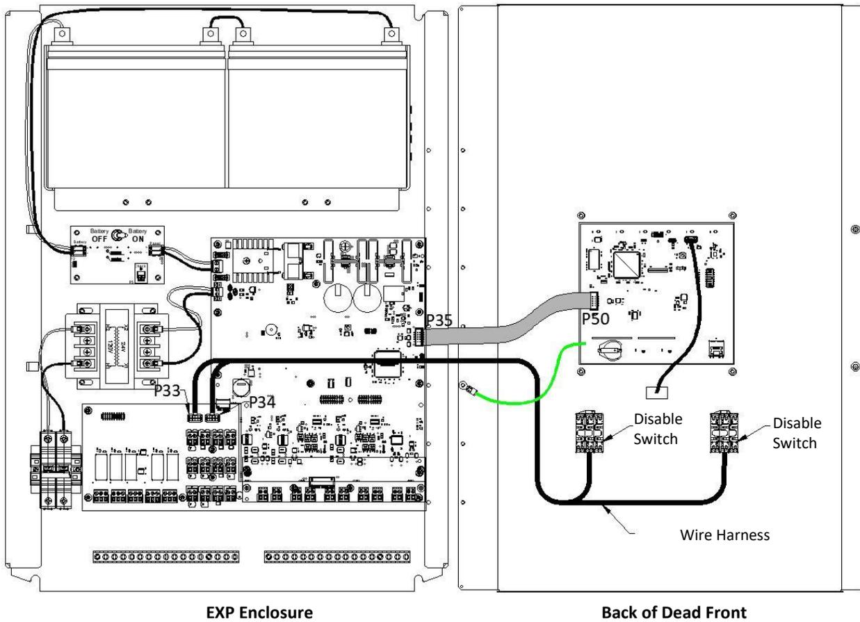
Figure 45 – Panel-Mounted Zone Disable Switch Wiring
