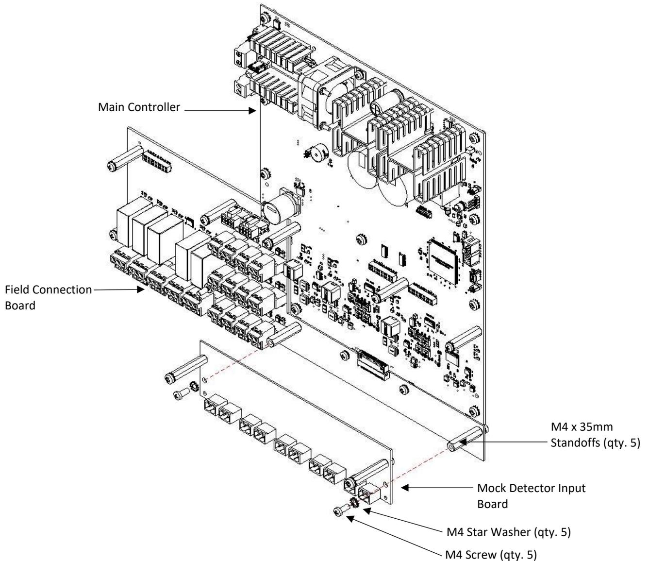
**Step 9.** Remove the screws and star washers (qty. 5) from the standoffs installed on the Main Controller Board and the Field Connection Board for mounting the Detector Input Board. See **Figure 234**.
