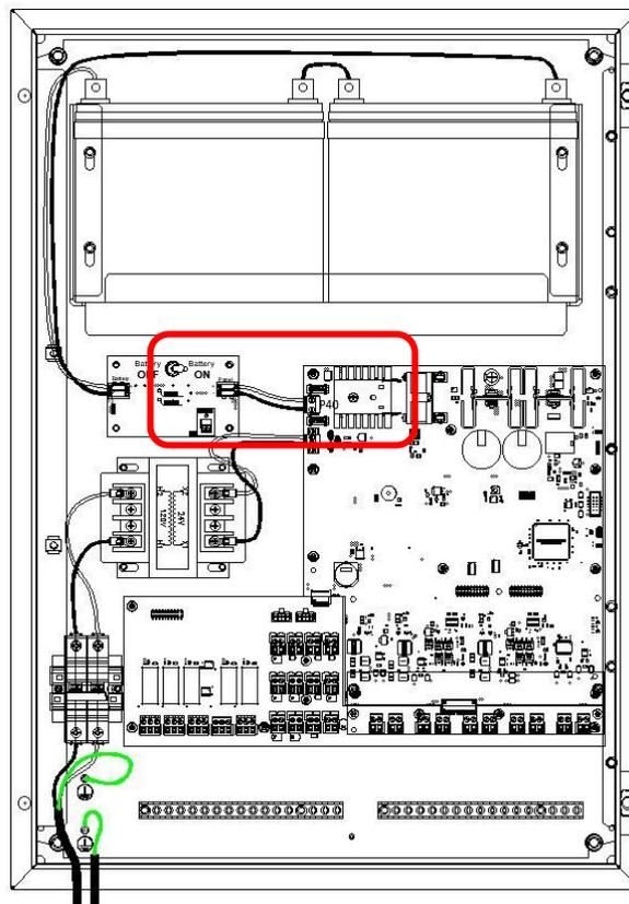
**Figure 42 – Standby Battery Connections**
