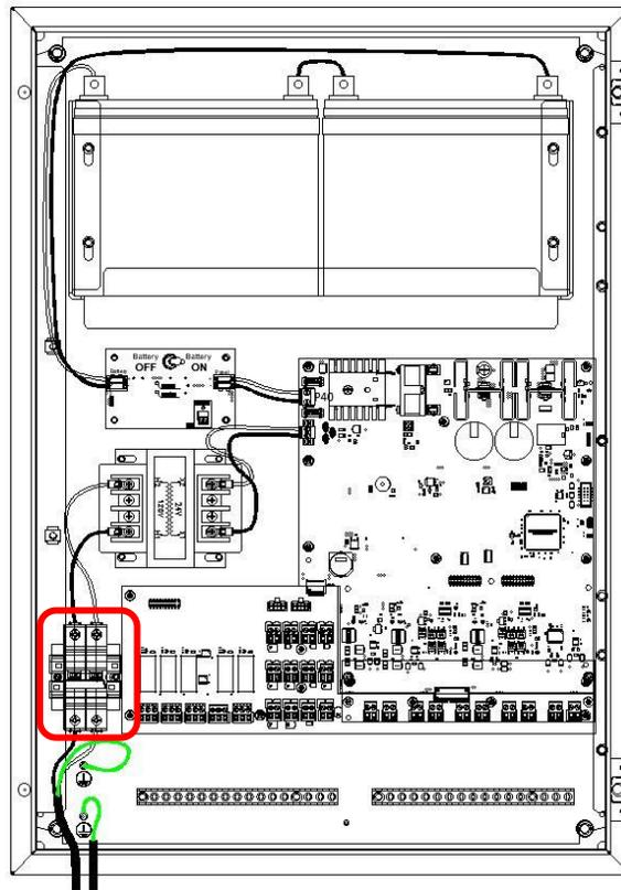
**Figure 38 – AC Line Power Connection**
