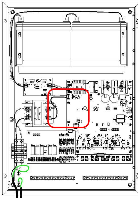
**Figure 40 – 24VAC Power Connection to Main Controller**
