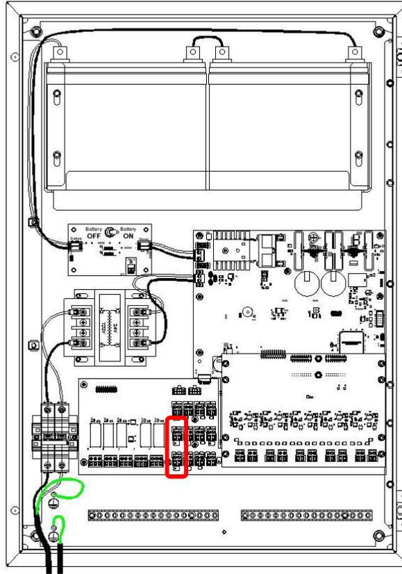
Figure 50 – Auxiliary Power Wiring (A, B, C)
