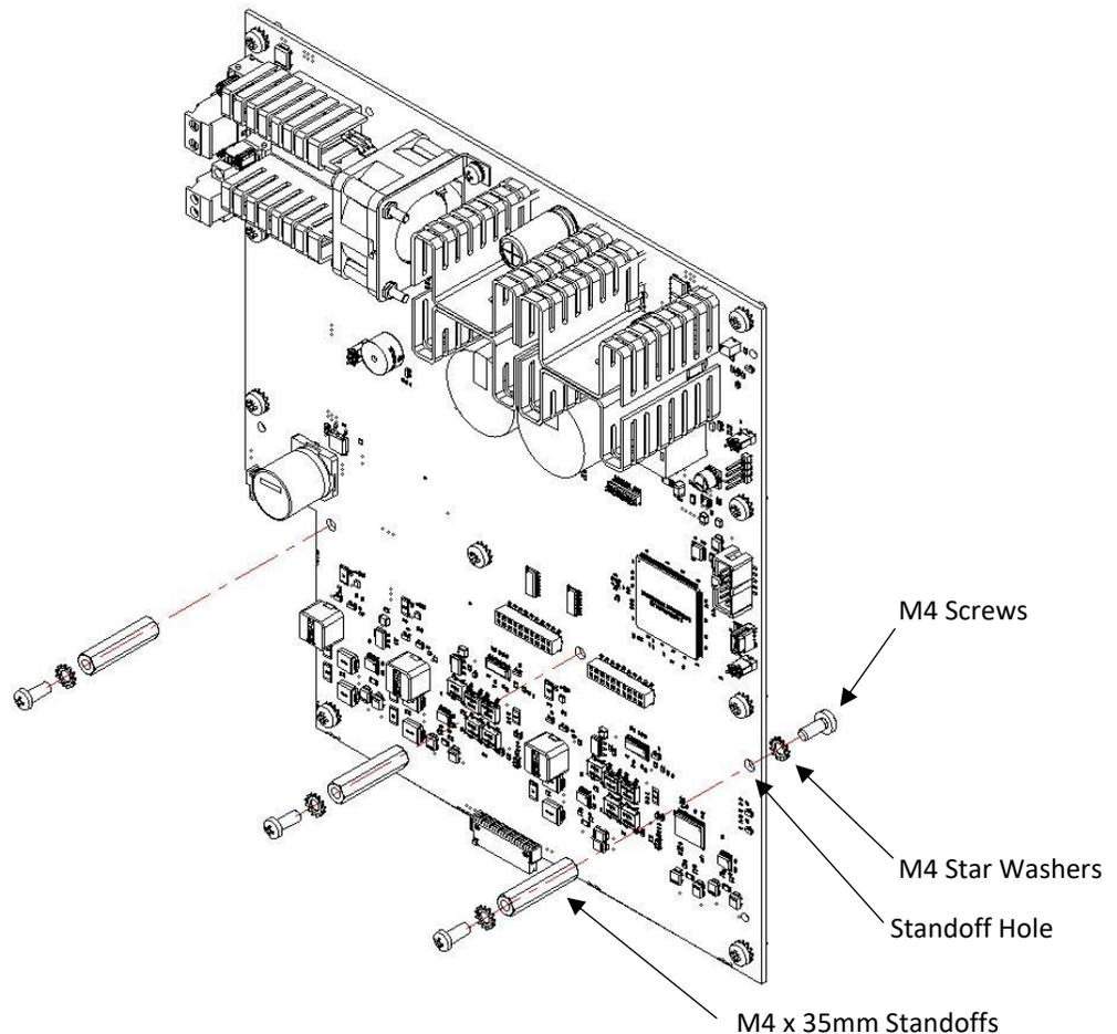
**Step 2.** Align the header connectors on the Main Controller with the mating connectors on the Field Connection Board, and gently connect the two boards. Verify that the headers are firmly seated. **See Figure 22.**
