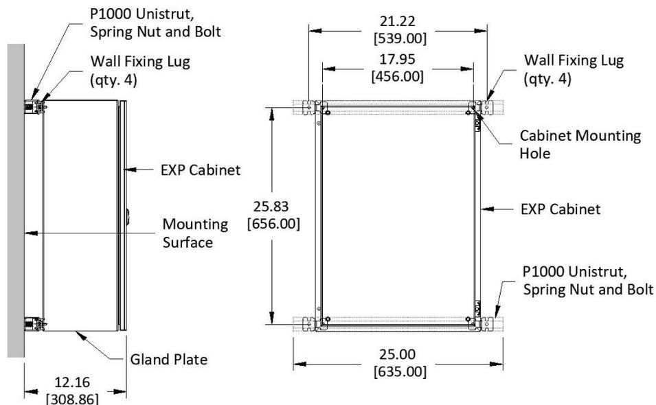
**Figure 20 – Fixing Lug Attachment to Channel (Schneider Lugs Shown)**
