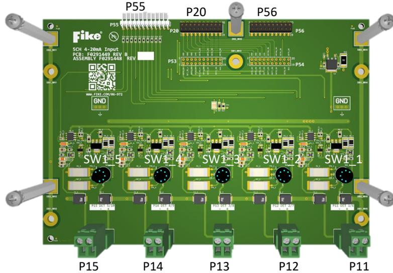
Table 10 – Class B, Non-Intrinsic Safe, Detector Input Board Components
