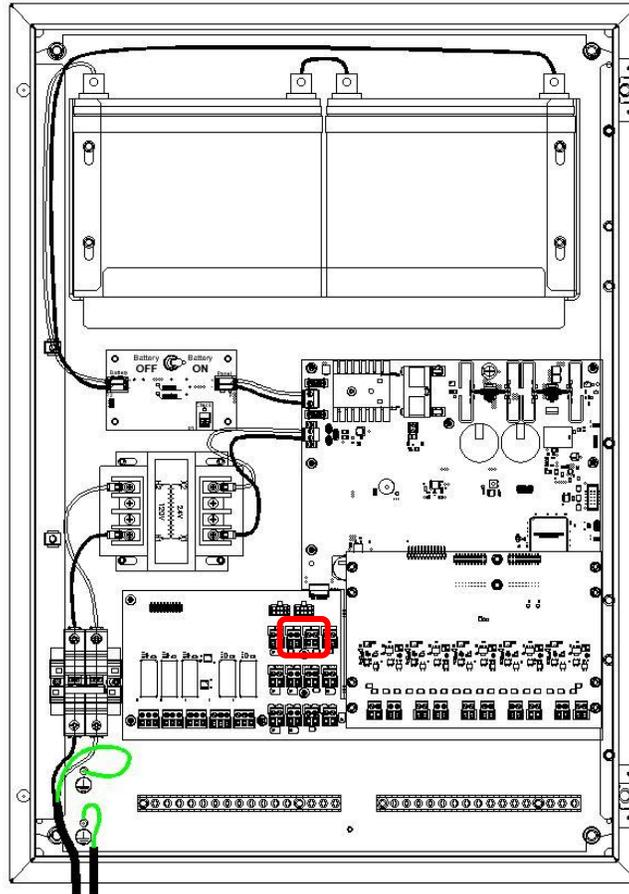
**Figure 57 – Remote Bus (Panel-to-Panel) Communication Wiring**
