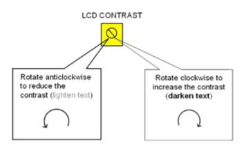
The LCD contrast may be adjusted by rotating the screw on the variable resistor, located in the upper right of the main PCB.
