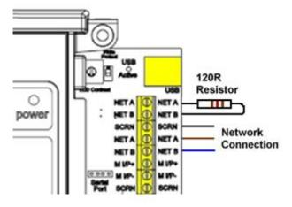
On the repeater a  $120\Omega$  Smoothing resistor must also be fitted across A and B but only on the last repeater on the network.
