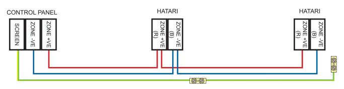
The Twinflex Hatari Sounder can be mixed on the same zone as other types of Twinflex device (eg. Twinflex Multipoint Detectors). The above diagram shows how to make the zone positive, zone negative and screen connections between the control panel and Twinflex Hatari Sounders. Refer to the instructions leaflets of other Twinflex devices for their equivalent wiring/terminal labelling details.
