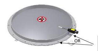
Install EM-BI-II burst indicator at NON-OPENING SIDE
