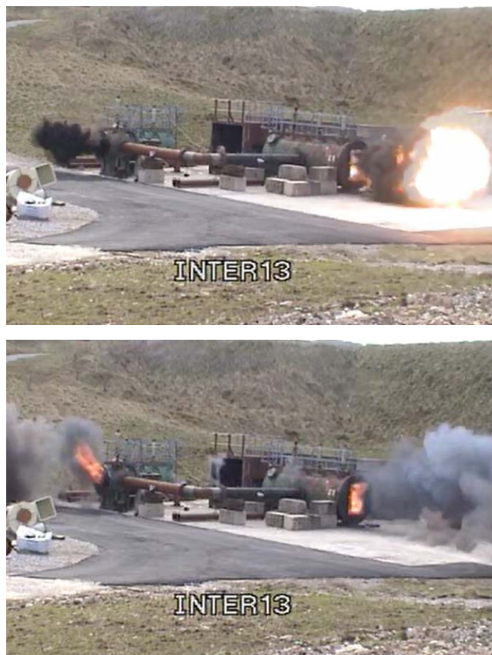
Figure 1. Interconnected vented vessels explosion tests performed by Health and Safety Laboratory (UK)
