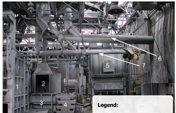
Figure 3. View of the dust collector (outside) and the facility (inside) after the dust explosion
