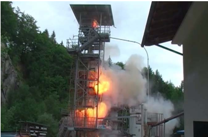
Figure 4. Dust explosion propagation tests performed by FSA (Germany)
