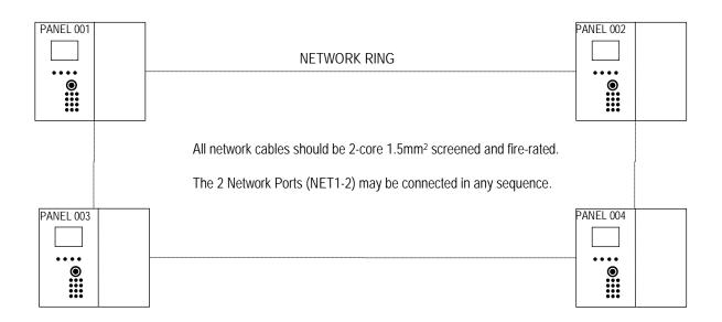
As shown above, the numbering of panels may be in any order. However, when planning an installation, it would make sense to number the panels sequentially in the order in which they are wired. The maximum number of networked units is 4. These can be a mixture of repeater panels and control panels.
