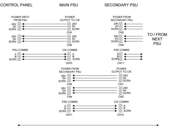
Total cable length from control panel to last PSU to be within specified limits for cable type depending on use of 1.5mm<sup>2</sup> or 2.5mm<sup>2</sup> cable for power.
