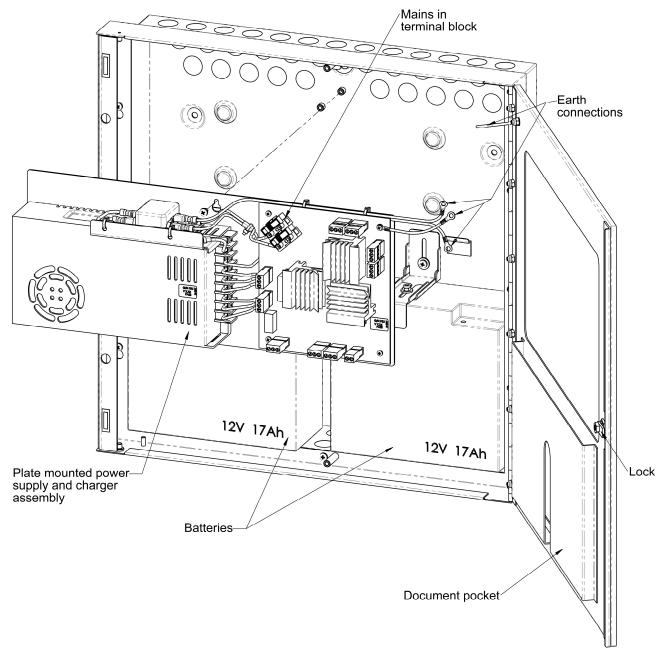
NOTE: The diagram above shows a V3 PSU. Earlier models differ slightly.
