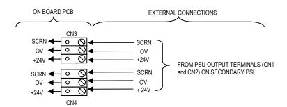
The Secondary PSU must be installed adjacent to the main Power Supply unit. Two 2-core 1.5mm<sup>2</sup> or 2.5 mm<sup>2</sup> screened cables should be used for the +24V and 0V power connections. These cables should be connected to earth at each end at the SCRN terminals provided
