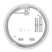
The Loop IN +ve (positive) and the Loop OUT +ve (positive) connections are split within the module. For cable continuity readings at the commissioning stage they must be temporarily removed and connected through. Please remember that all high voltage testing must be carried out before the installation of the electronics, otherwise the electronics will be damaged. Please also note that the SCRN terminal should only be connected to the loop screen and NOT the building earth.
