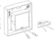
The MCP is installed by locating the upper mounting hook into the receiver in the back box and then pushing the unit gently home. The single fixing screw may then be tightened as required.
