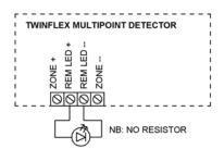
If a remote indication LED is required to indicate the operation of a Multipoint detector, you may connect as shown here.
