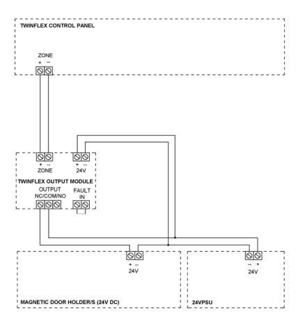
If this is not convenient, then the lower left diagram shows how to connect door hold magnets using the Twinflex Output Module.
