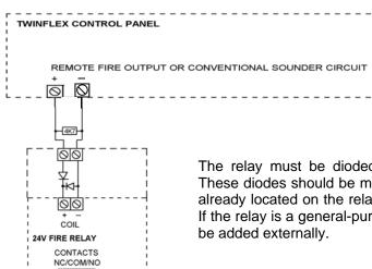
The relay must be dioded for polarisation and suppression as shown. These diodes should be marked 1N4001 or of a similar type, and may be already located on the relay PCB if it is designed for Fire Alarm Systems. If the relay is a general-purpose plug-in relay then the diodes may need to be added externally.
