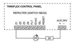
If a remote indication LED is required to indicate the activation of a zone at the control panel, then connect as shown here.
