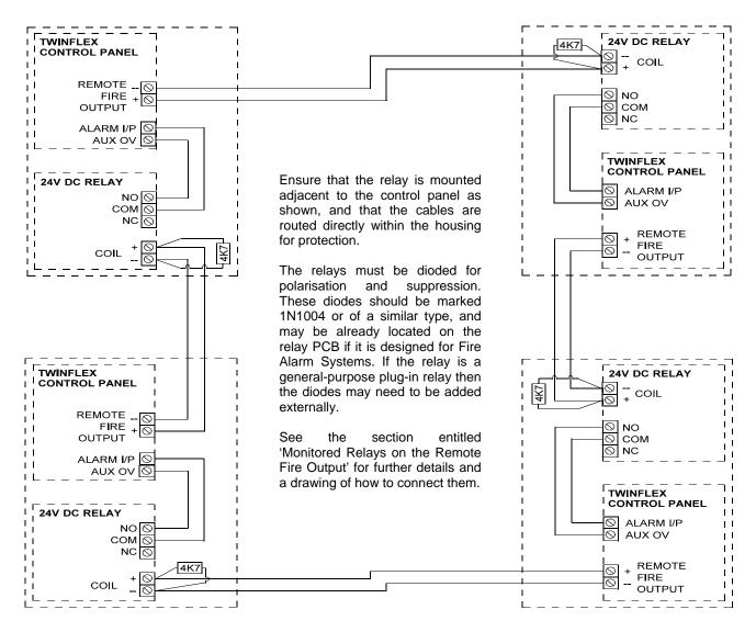
In order to interconnect a number of Twinflex control panels together connect them as shown above. This will ensure that all cables are monitored, and system lock-up will be avoided.
