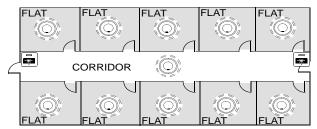
The Drawing below shows a larger apartment with several Multipoint detectors. The apartment should be cabled on its own zone and the Alarm Confirmation Alarm should be set to operate in a Zonal manner, so that all persons within the apartment are alerted.
