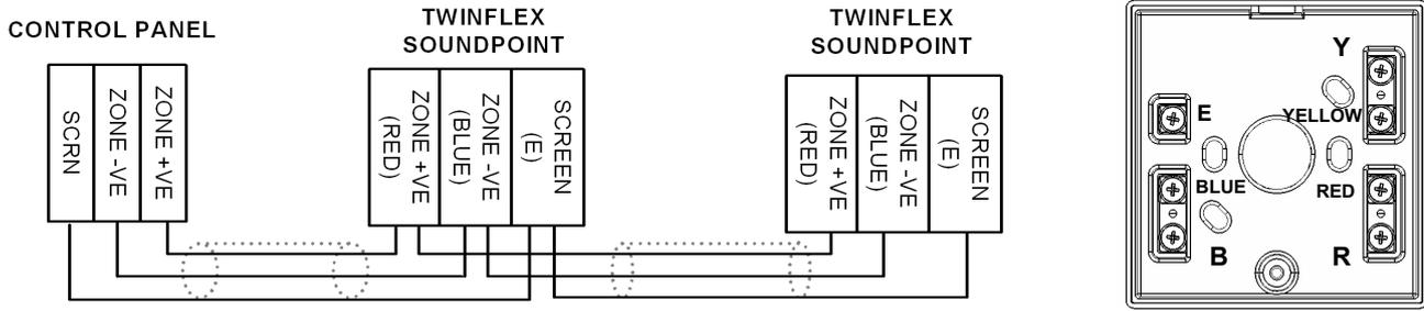
Twinflex Soundpoints can be mixed on the same zone as other types of Twinflex device (eg. Twinflex Multipoint Detectors). The above diagram shows how to make the zone positive, zone negative and screen connections between the control panel and Twinflex Soundpoints. Refer to the instruction leaflets supplied with other Twinflex devices for their equivalent wiring/terminal labelling details.
