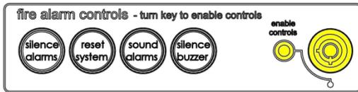
You may gain access to the fire alarm controls by inserting the key turning  $\frac{1}{4}$  turn. The 'Controls Enabled' LED should then be illuminated.
