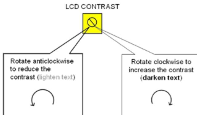
The LCD contrast may be adjusted by rotating the screw on the variable resistor, located in the upper right of the main PCB.
