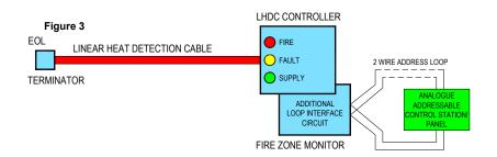
Notes: Configurations for Fig 2 & 3, is dependant on the voltage and current specifications of the LDM-519-LP being compatible with the monitoring technique and electrical characteristics of the Control Panel / Zone Monitor.
