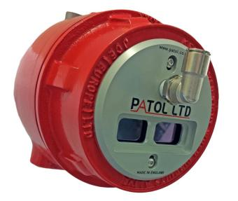
The 5000 Series is an early warning infra-red heat sensor, which can trigger at temperatures as low as 100°C, when monitoring materials being transported on conveyor systems, before they have reached the ember or flame condition.
