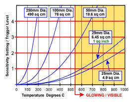
The chart (left) indicates the correlation between the temperature and size of 'hot spot' anomalies for a typical installation to produce one or more detector channel activations at various trigger level settings.
