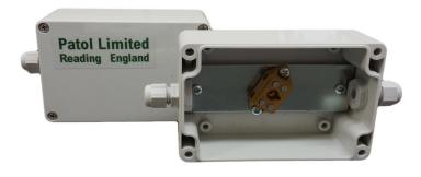
The Polycarbonate Junction Box is a basic method of jointing either Digital or Analogue LHDC and is supplied with two glands. It can also be used as a connection junction box between an interposing cable and the LHDC.
