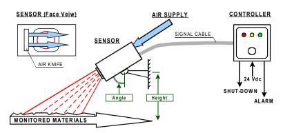
The sensor is located above or beside the materials transit path (conveyor, roadway, etc.) by means of the adjustable mounting bracket and aligned such that the monitored hazard passes through the sensor's field of view. The distance and angle of the sensor determine the width of the monitored path.
