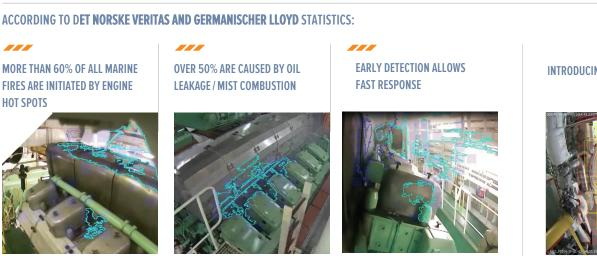
Effective oil mist detection with live video verification can provide early warning and allow quick response to avoid fire or explosion.
