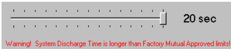
Extended discharge times can be used for retrofitting certain Halon 1301 systems. Always try to run a flow calculation using the Normal discharge time of 10 seconds. If 10 seconds is not long enough to flow HFC-125 through your Halon pipe network, you may extend the discharge time out to 20 seconds.
