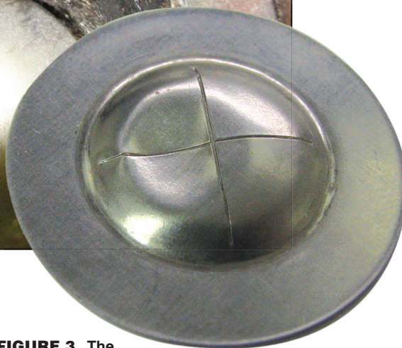
FIGURE 3. The damage on this forward-acting rupture disc is a result of freezing condensate
