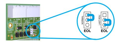
The jumpers are fitted to impedance match the cable with the driver ICs & prevent signal reflections down the cable. The jumpers <u>must</u> be changed on the **CIE** and last **RDU**.
