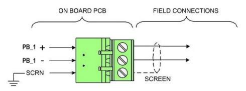
Communications between the panel and repeater is via a multi-drop RS-485 Peripheral Bus. 2-core 1.5mm<sup>2</sup> screened fire resistant cable (i.e. FP200, Firetuff, Firecell) cable should be used for communications to the repeater.
