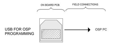
The CIE-A-200 control panel may be programmed using the CIE-A-200 OSP programming software with a USB lead to link the User USB port to a computer. This allows the site specific data to be customised as required.
