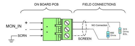
Maximum Voltage at contacts, 3.3 Volts. Maximum current 10mA. Monitored Inputs 1 & 2 will monitor for open and short circuit faults using a 3k3 EOL resistor. To activate the input, connect a 680R or 470R 'triggering' resistor across + & -.
