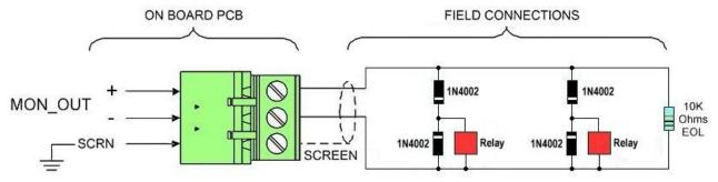
The default setting for monitored output 1 is a **Monitored Sounder Output** and the default setting for monitored output 2 is a **Common Fire Output**.
