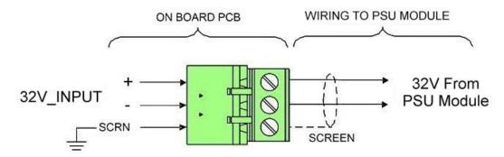
The panel requires a DC supply voltage of 27.5V - 33.5V which is supplied by the internal 150W switch mode PSU module.
