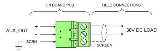
An auxiliary nominal 24V DC power supply is available to power ancillary devices requiring up to 30V DC. The maximum output current is **450mA**. The Auxiliary Power output is protected by **T500mA** fuse F1.
