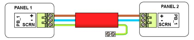
The peripheral bus must be run from the panel to the first repeater then the second repeater and so on; the peripheral bus must not be spurred from one point.
