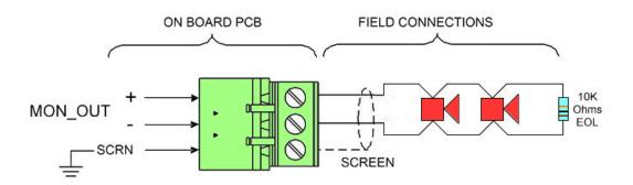
Outputs 1 and 2 are monitored circuits which are monitored for open and short circuit faults with a 10k EOL resistor. Sounders used on monitored outputs must be 24v conventional type sounders.
